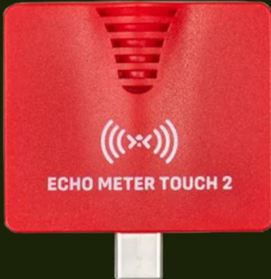
The “Echo Meter Touch 2” unit plugs into a tablet or phone. It is a microphone capable of detecting the high frequency sounds that bats make. Devices need the **free “Echo Meter Touch Bat Detector” app** for the unit to function. Using the device and app, you will **hear** a modified version of bat’s echolocation calls, and **see** a visual representation (**spectrogram**) of this sound.
